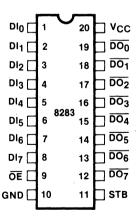
Figure 2. 8283 Pin Configuration
